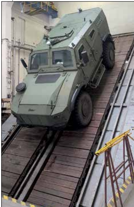
■ In testing the effectiveness of the parking brake system, the Gerlach achieved a slope of 83.9%.
