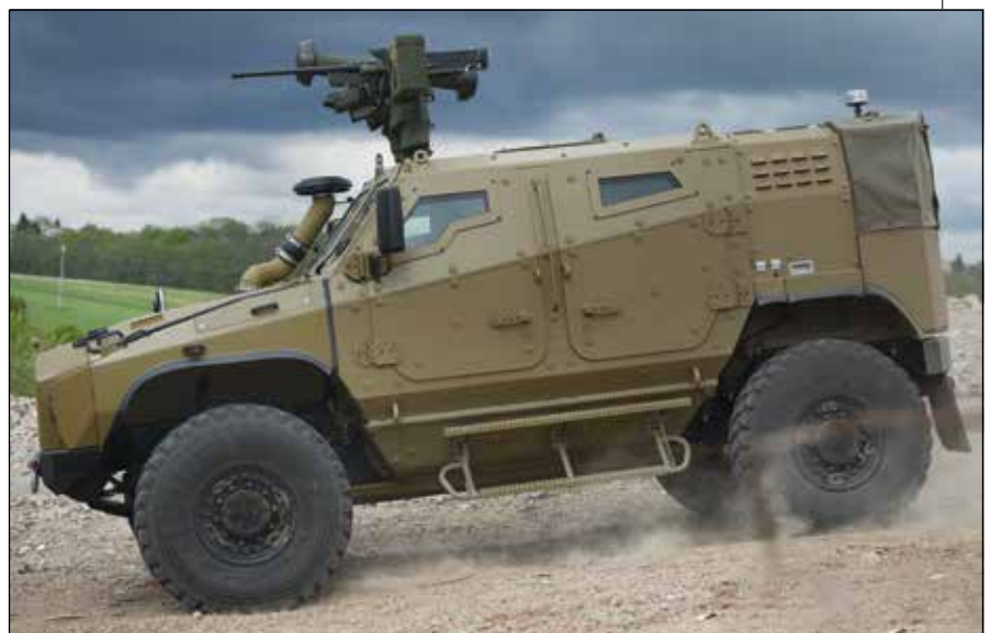
■ Special chassis, massive torque and ground clearance of up to 465 mm ensure the vehicle's excellence in terrain
