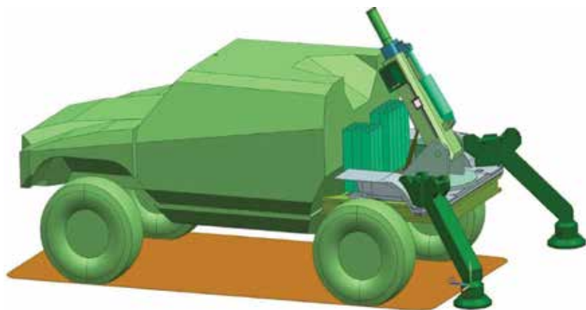
■ 120 mm guided mortar with built-in hydraulic supports and reinforced frame
